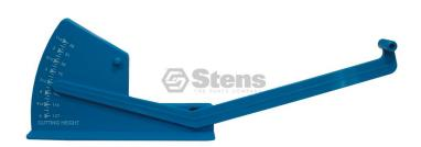
Leveling Gauge Plastic PlasticUsed to accurately level and measure mower decks on all riding and walk behind mowersMower blade cutting height gauge range is 1 1-2" to 5"Measure tip to tip cutting edge (side to side and front to back)- Measure one side cutting edge. Check height on gauge.- Measure other side cutting edge. Check height on gauge.- Deck is level if heights are the same. If not, deck adjustments will need to be made.USE GLOVES TO AVOID INJURY
