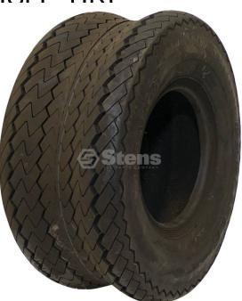
Tread: Links Tread Links Tire Size 18x8.50-8 Ply 4 Rim Size 8" Max PSI 22 Max Load Capacity 825 Type TubelessCarry their loads without wear and tear on the turf or fairway and ride smoothly on paved pathsWork well as wide-flotation tires for on-site transport on heavy-duty jobsProven rubber compounds and tread designs get the job doneTire and wheel solutions for homeowner and grounds care professional applications Use with 170-084 Tube 170-084 Tube
